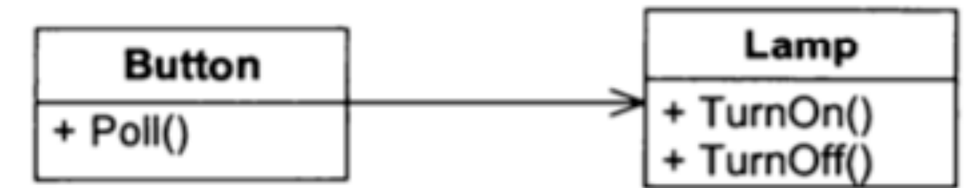
Figure 11-3 Naive Model of a Button and a Lamp
