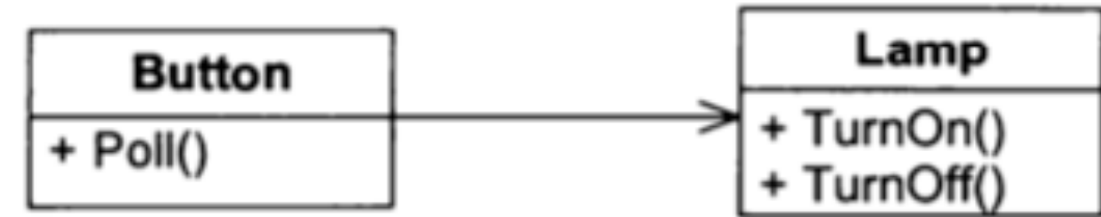
Figure 11-3 Naive Model of a Button and a Lamp
